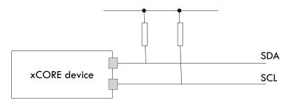
Figure 1: I2C open-drain layout
